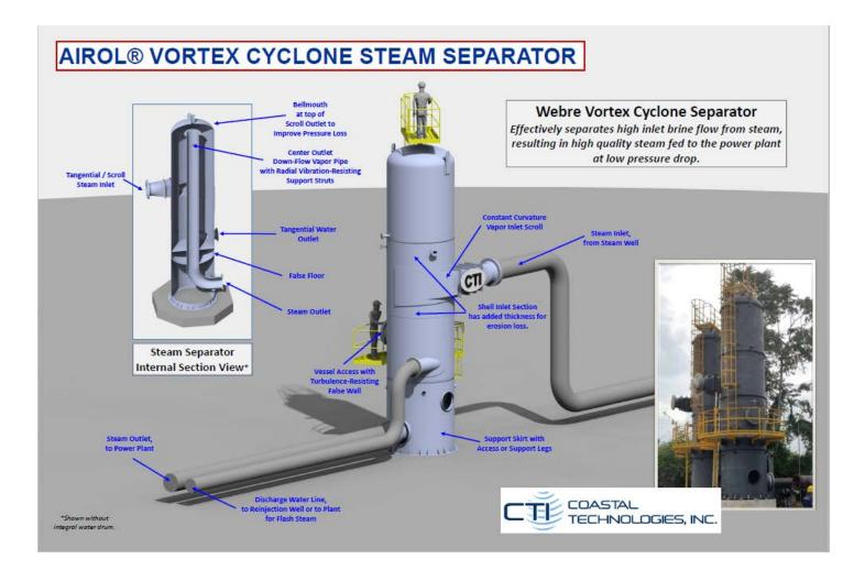
Water and steam is forced into circular cyclonic motion as a result of the mid-level tangential constant curvature inlet. Water spirals downward toward the tangential water outlet at the base. Steam spirals upward with centrifugal force moving remaining droplets to the side walls, where it drains down to the base. Steam continues to cyclonically spin to the top where it reverses flow and moves down the steam outlet pipe.
