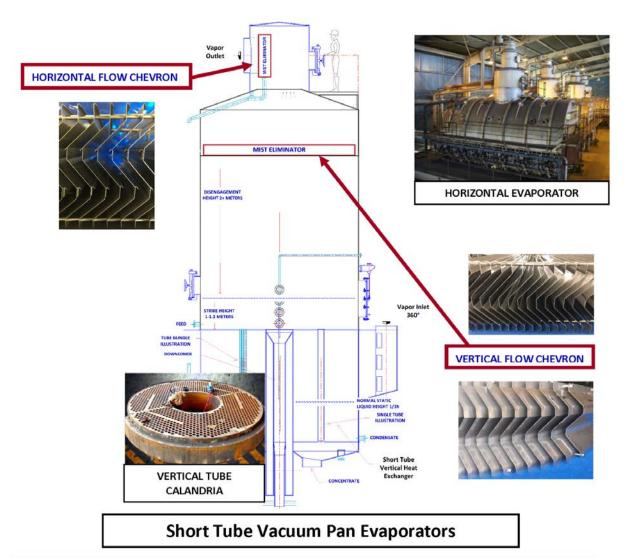
Material flows through tubes heated by low pressure steam condensing on the outer tube surface. The boiling liquid is under a moderate vacuum, which reduces its boiling point, thereby increasing the heat transfer rate in the evaporator.
