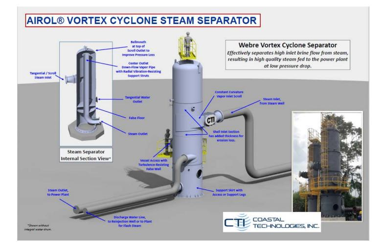
Water and steam is forced into circular cyclonic motion as a result of the mid-level tangential constant curvature inlet. Water spirals downward toward the tangential water outlet at the base. Steam spirals upward with centrifugal force moving remaining droplets to the side walls, where it drains down to the base. Steam continues to cyclonically spin to the top where it reverses flow and moves down the steam outlet pipe.
