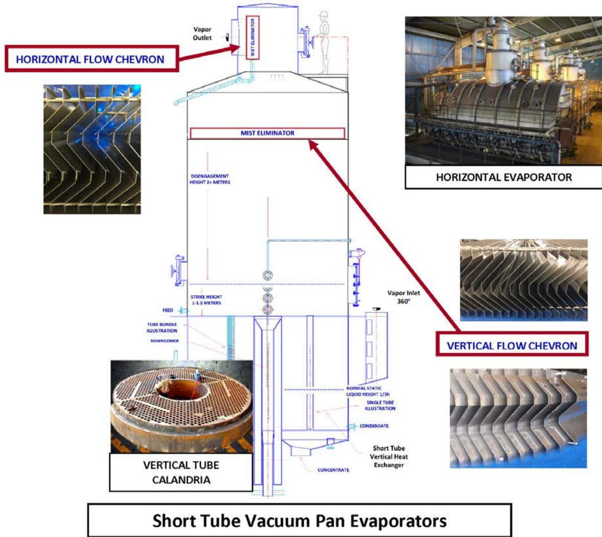
**Short Tube Vacuum Pan Evaporators**
