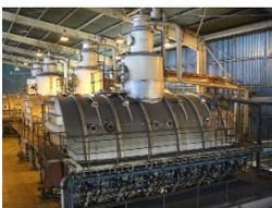
A popular evaporator in the US has been the horizontal tube type, in which the tube bundle is located in a rectangular heat exchanger. As with the vertical evaporator tubes, the sugar solution flows through the inside of the tubes. In horizontal tube design heat exchangers, liquor circulation is not as robust so, generally, they are not used with viscous liquids.
